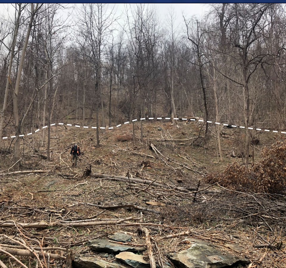
Photograph: weathered concave headscarp with piles of subangular-to-angular bouldery debris. These features are often found within colluvial hollows or along linear tracks.
