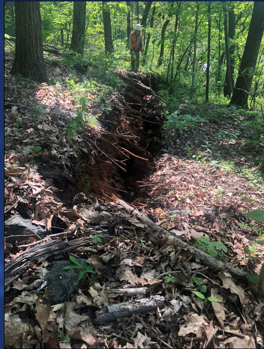
Large tension crack in soil. This indicates the ground is shifting.
