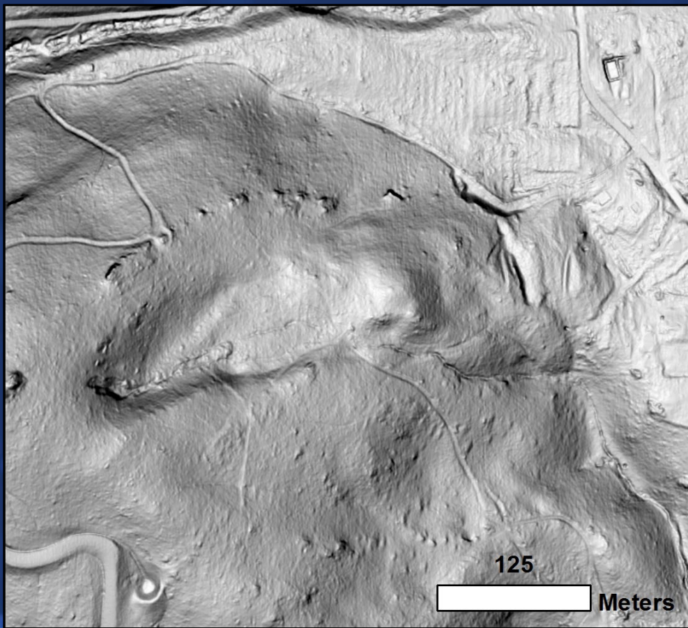
Weathered Landslide: headscarp and lateral edges weathered but identifiable in LIDAR; cannot be associated with a storm event.
